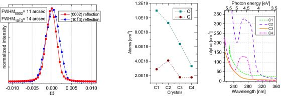
Fig.1: Rocking curves (open detector) measured with 4-bounce Ge220 monochromator
